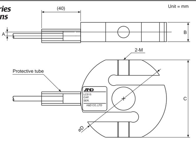
\* When used with stainless steel rod-end bearings, please ensure that the normal operating load is less than 1/2 of the rated capacity of the load cell.
